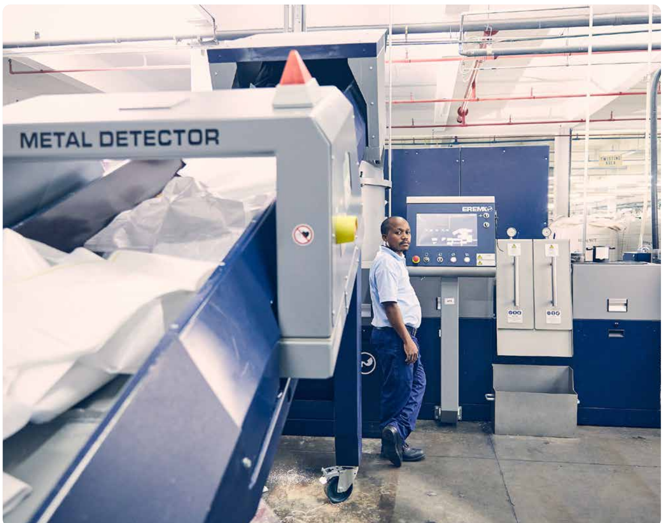
Polypropylene Products: Recycling machine that recycles the polymer waste, off cuts and rejects.
