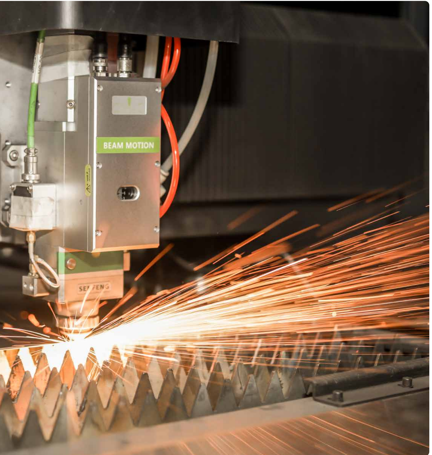
Premier Rainwatergoods: Fibre laser machine cutting light steel.
