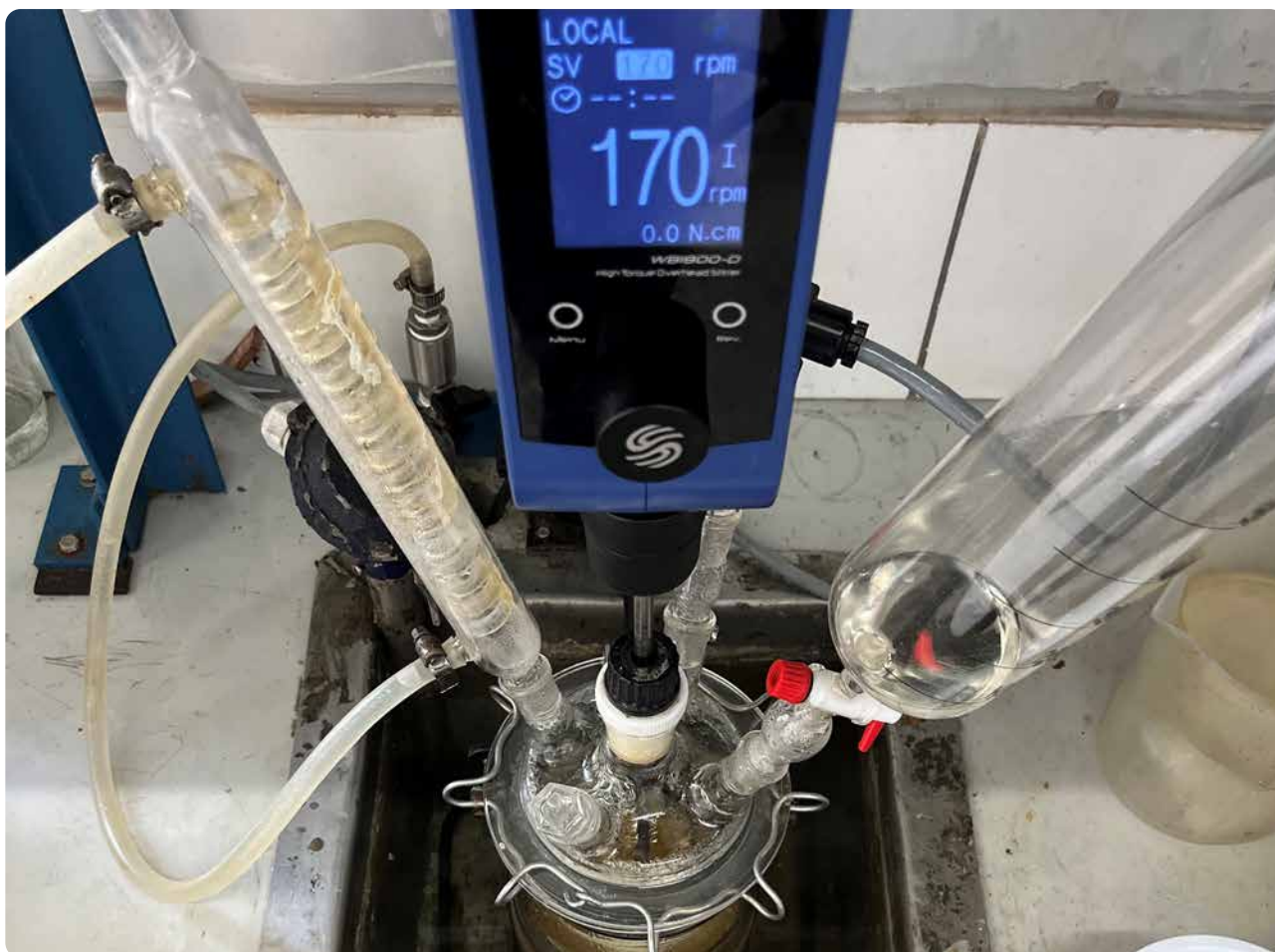
Gold Reef Speciality Chemicals: Laboratory reactor used for polymerising products in the lab.
