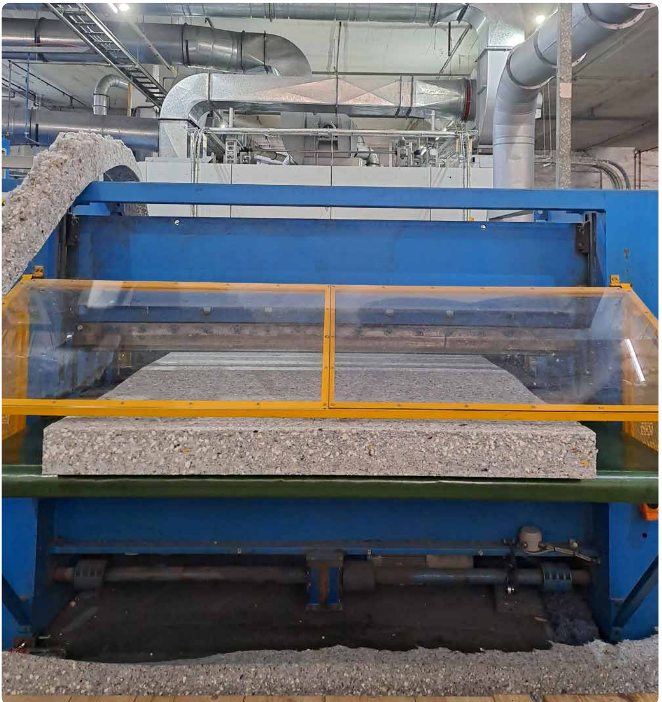
Brits Nonwoven: Airlay line production of recycled mattresses.
