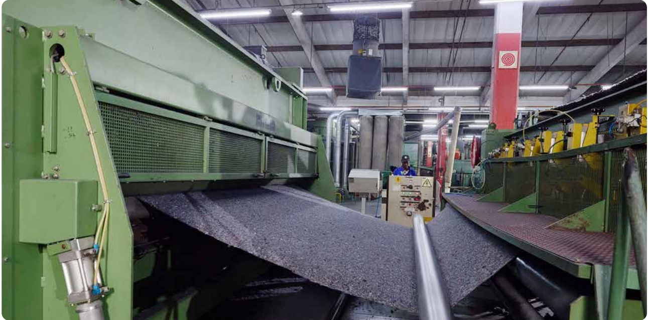
Brits Nonwoven: The manufacture of felts using needle punch technology.
