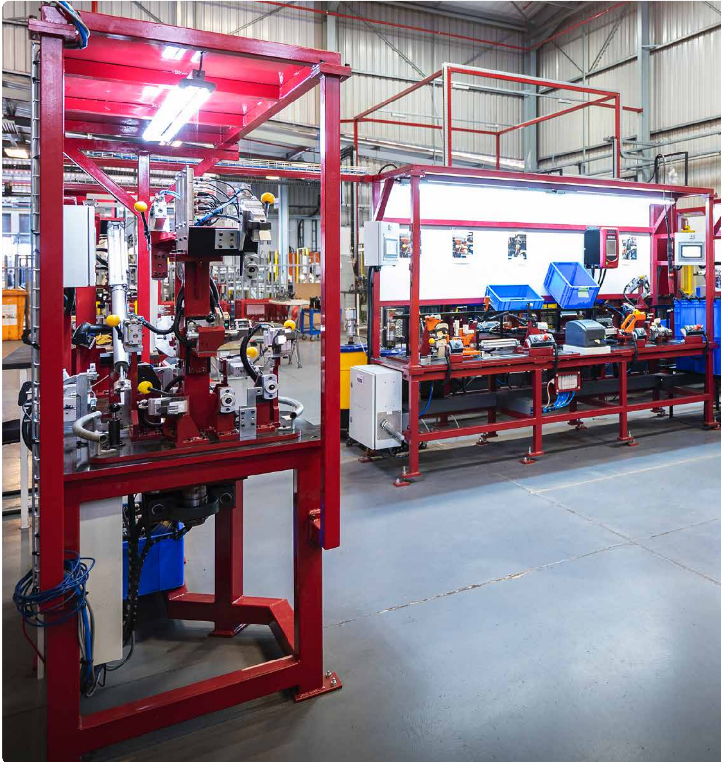
Formex: Assembly of Ford Ranger Clutch and Brake components.
